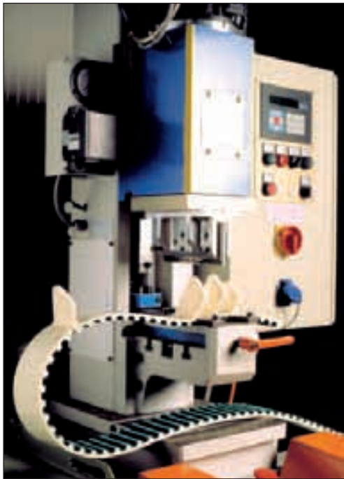
Cleat welding machine
